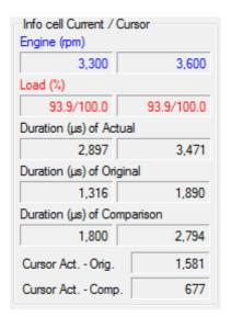
This panel shows the value(s) of the cell(s) that have been selected with the cursor. It displays also the RPM and the load range of the selected cell.
