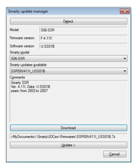
The "**Detect**" button verifies which Smarty is connected to the PC and selects it form the drop down menu. In addition, the most relevant parameters like firmware revision and level are displayed.
